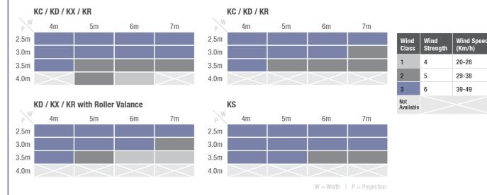
Awnings must be mounted with the right amount of installation brackets and with suitable fasteners in order to match the specified wind classes. Ideally Kona Awnings should be fully retracted during high winds.
